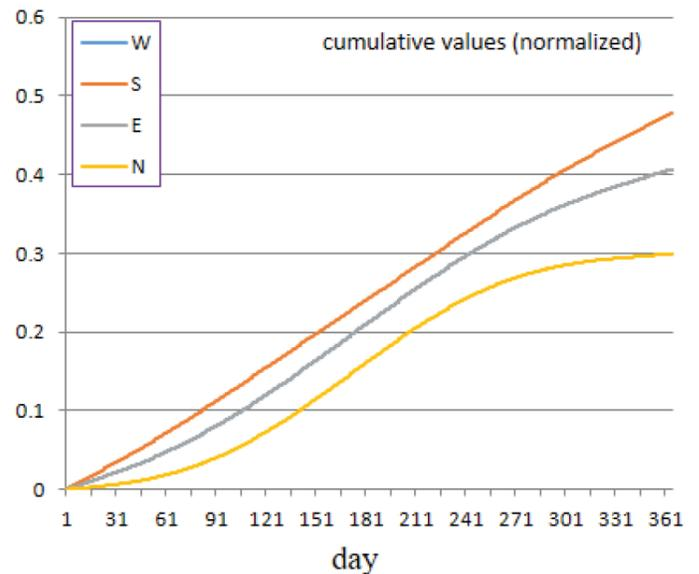
**Fig. 2:** Numerical examples. Daily behaviours of  $\cos\theta$  for a window of 365 days: daily and cumulative (normalized) for West, East, North and South-facing scenarios. East and West scenarios are equivalent for symmetry under our examination settings.
