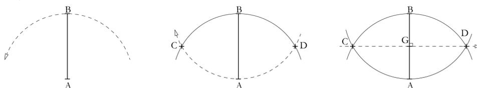
Draw a perpendicular line or find the middle of a given segment: **3 steps**
