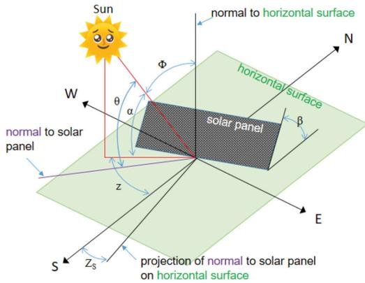
**Fig. 1:** Solar angle diagram for modeling the incidence angle  $\theta$  for a solar panel.
